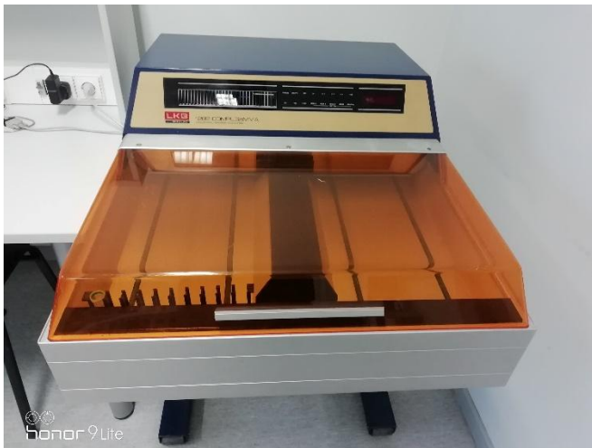
Fig. 1. Gamma spectrometer “CompuGamma 1282” spectrometer
