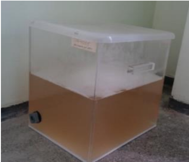
Gelatine based phantom, for noise sample generation.
